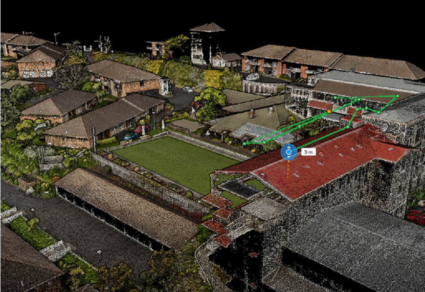
Pictured: Point cloud generated from survey drone used as base map for spray route planning.
